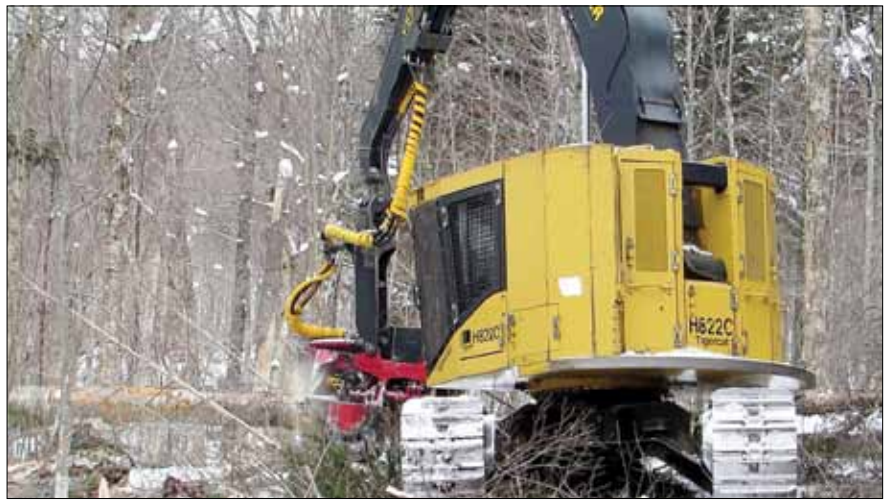
A Tigercat harvester with small tail swing. Tolerance for damage to retained trees is another factor that the landowner should negotiate with the contractor before work proceeds.
