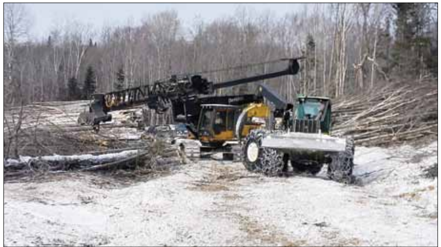
The traditional full-tree harvesting system, based on roadside processing, is still used, though cut-to-length harvesters have become more common.
