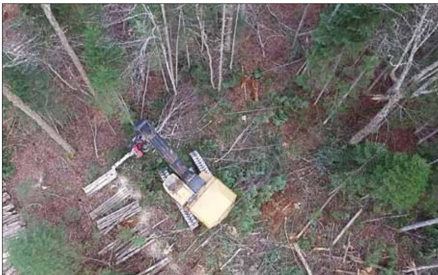
Tracked harvester with large tail swing. On any forestry treatment, the choice of equipment to be used is at the landowner's discretion.
